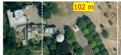
The Airy meridian (dashed line) and the ITRF zero meridian (solid line). Imagery© 2014 Google Maps, Infomars Ltd & Bbecky
